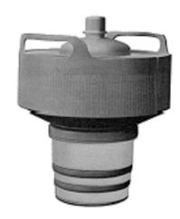
The YC-130 broadcast tetrode is externally identical to the 4CX15,000A/8281. Internal construction features a mesh filament and Y-3 wire grids. The mesh filament is particularly well suited to FM service at 108 MHz due to reduced filament inductance. The YC-130 filament operates at 7.5 volts.
